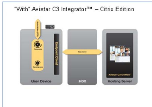
Using this architecture, the Citrix-enabled Avistar C3 Media Engine™ solution plugs into application software running on the server using the exact same interfaces as those of the standard media engine, but all interface requests are relayed to the client-based media engine module using the Citrix HDX protocol.
